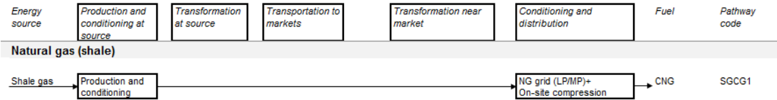
Figure 11. Natural gas (shale gas) pathway
